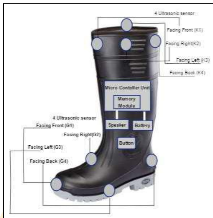
Fig 1. Smart Shoe system showing arrangement of system components
