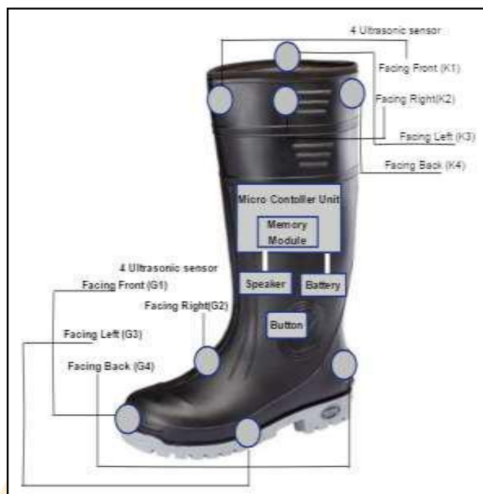
Fig 1. Smart Shoe system showing arrangement of system components
